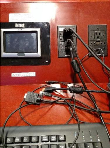
Attach your laptop to the podium via the cables on top. Connectors for picture, sound, and network are provided. The top video connection is for the laptop. The bottom video connection is for the ELMO document camera.
